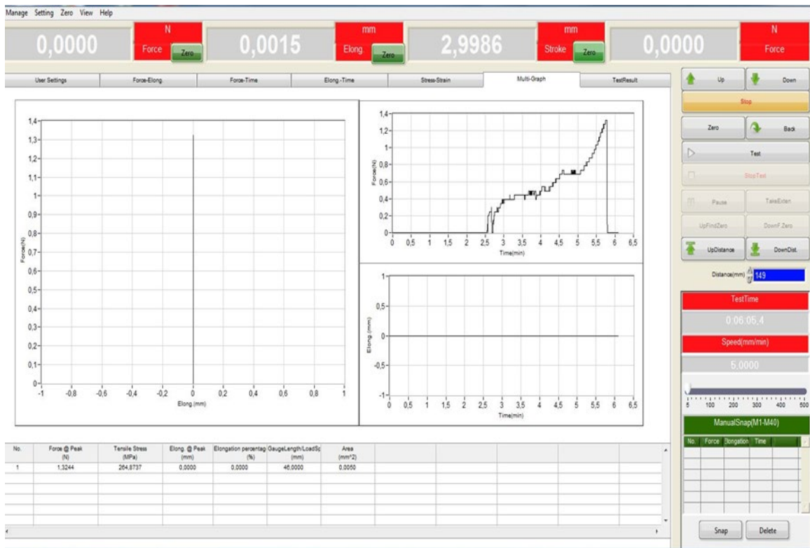
Figure 8. Result of fiber breakage after pull out
